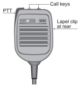
Either of the 2 call keys on top of the speaker-microphone can be used to initiate a call. On T3030, T3035 and T3040 trunked handportables, this feature is available if the radio has been programmed with the 'external call request' facility.
